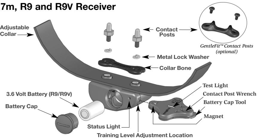
The components of both the R9 and R9V (above) and the R7m are the same except the R7m is smaller and uses a different battery.
