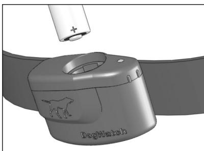
Insert R9/R9V battery POSITIVE end down.
