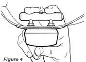
**Test Light:** The test light allows you to test the receiver. Hold the test light over the contact posts. (Figure 4) and carry the receiver into the signal field. When the receiver picks up the signal from the boundary wire, the audible warning will sound and the test light will come on.
