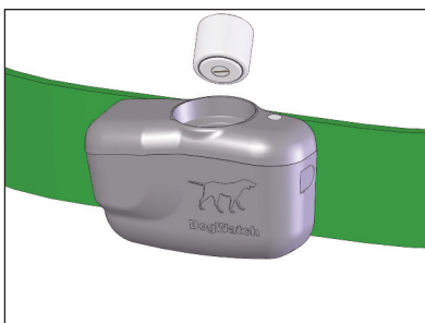
Insert R7 battery NEGATIVE end down.
